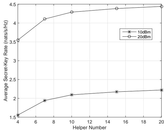
**Figure 7.** Average secret-key rate versus helper number for Rayleigh fading channels with total transmitting power of 10 dBm and 20 dBm.
