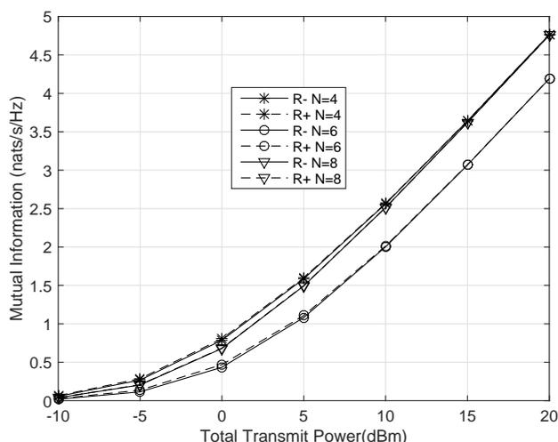
Figure 5. Upper and lower bound of secret-key capacity with the channels listed in Table 1. In the figure,  $R^+$  and  $R^-$  are close to each other, which verifies the result of Theorem 1.
