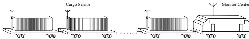
**Figure 1.** System Configure. In the system, cargo sensors (CS) are placed on the cargo containers to monitor or secure the containers. The monitor center (MC) is normally placed in locomotive. MC communicate with CS through wireless link, which should be secured by cryptography algorithm.
