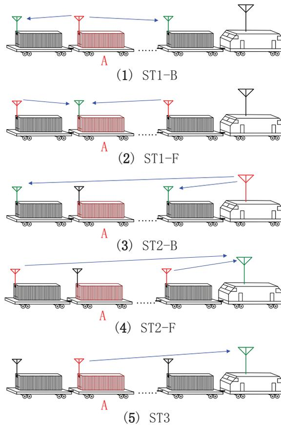
**Figure 3.** Algorithm steps. (1) A sends channel estimating sequence to helpers; (2) helpers transmit random signals simultaneously to A; (3) MC sends channel estimating sequence to helpers; (4) helpers send reversed random signals simultaneously to MC; (5) A communicates with MC to get agreement on the secret-key. Note that in the figure when sending signals the antenna is colored in red, when receiving signals the antenna is colored in green.
