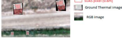
**Figure 8.** Example of ground temperature images georeferenced from locations shown in Figure 6 and others over a visual image using ArcGIS. The figure showcases thermal temperature images of two bare soil locations (top) and two tall canopies (vines) (bottom). Square grids indicate sUAS and ground pixels that can be extracted for atmospheric radiance calibration.
