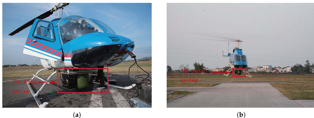
Figure 7. The Ka bandwidth radar system and helicopter platform. (a) The Ka bandwidth radar system. (b) The helicopter platform.
