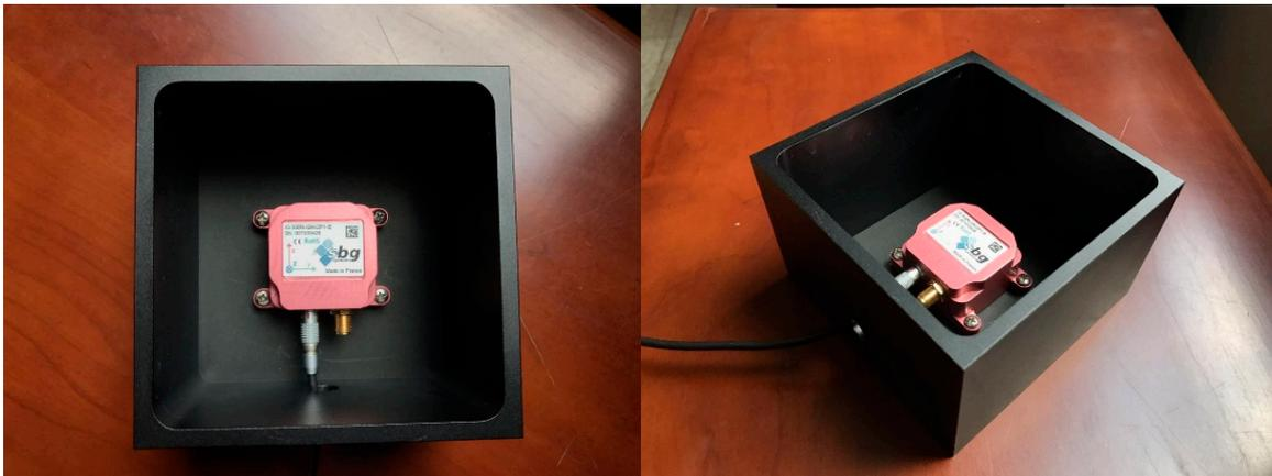
**Figure 9.** Cuboid frame with the mounted sensor set.
