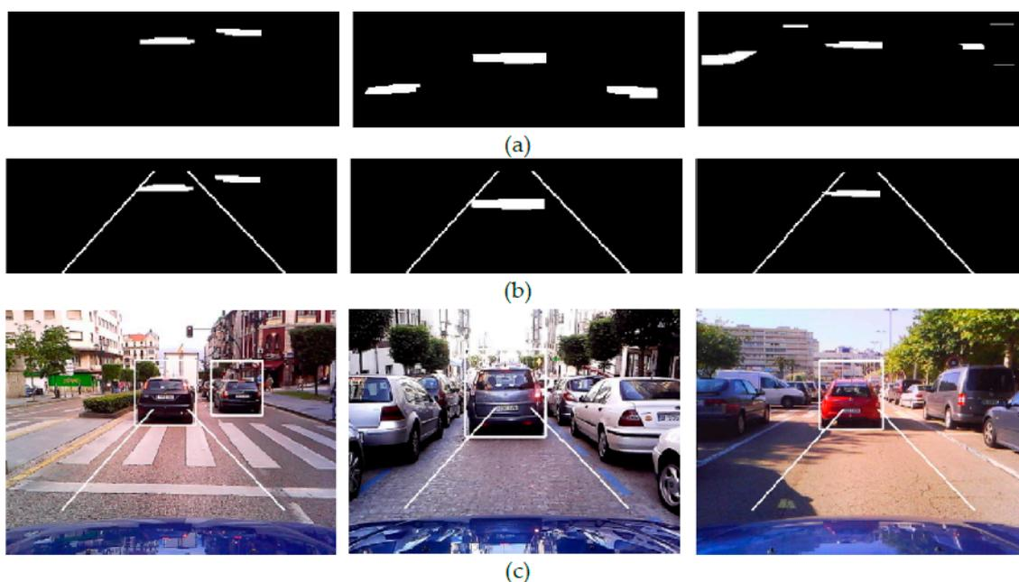
**Figure 5.** (a) Binary mask  $M(x, y)$  of Figure 2 after horizontal clusters extraction (b)  $M(x, y)$  after morphological thresholding and ROI establishment; and (c) vehicle hypotheses including those out of the ROI.
