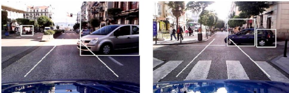
**Figure 7.** Hypotheses generated by vehicles travelling transversely on crossroads.
