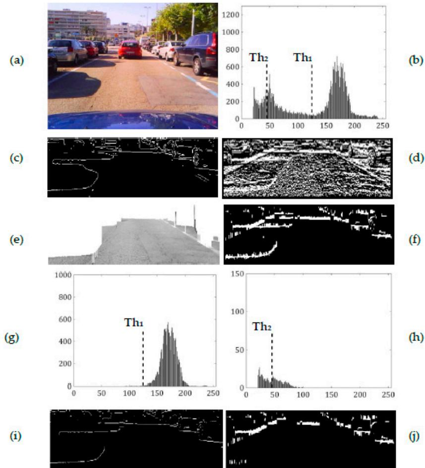
**Figure 10.** Road scene on a sunny day. (a) searched image area, (b) its greyscale histogram. Left column (method proposed in [21]): (c) edge map, (e) free driving road, (g) histogram of the free driving road and (i) edge map after intensity thresholding. Right column (our method): (d) vertical intensity gradients, (f)  $M(x, y)$  after application of saturation and intensity constraints, (h) histogram of set of upper pixels of the gradients and (j)  $M(x, y)$  after intensity thresholding.
