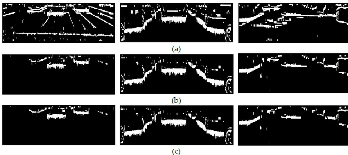
**Figure 2.** (a) Binary masks  $M(x, y)$  of Figure 1 after application of the saturation and intensity difference constraints, (b)  $M(x, y)$  after intensity thresholding and (c)  $M(x, y)$  after extraction of adjacent gradients due to lateral shadows.
