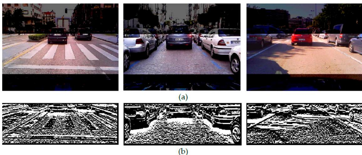
**Figure 1.** City centre roads with road markings, vehicles parked on both sides and cluttered backgrounds in overcast and sunny conditions. (a) Searching image region (b) vertical intensity gradients  $M(x, y)$ .
