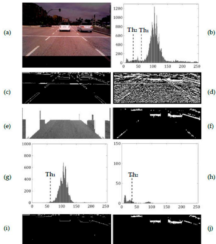
**Figure 9.** Road scene on cloudy day. (a) Searched image area; (b) its greyscale histogram. *Left column* (method proposed in [21]): (c) edge map, (e) free driving road, (g) histogram of the free driving road and (i) edge map after intensity thresholding. *Right column* (our method): (d) vertical intensity gradients, (f)  $M(x, y)$  after application of saturation and intensity constraints, (h) histogram of set of upper pixels of the gradients and (j)  $M(x, y)$  after intensity thresholding.
