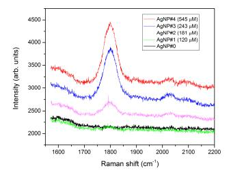
Figure 7. Raman spectra of AgNP colloidal solutions with different glyphosate concentrations.
