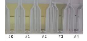
**Figure 5.** Picture of different colloidal solutions with increasing glyphosate content from left to right: AgNP#0 (pure citrate capped silver nanoparticles), AgNP#1 (120 µM of glyphosate), AgNP#2 (181 µM of glyphosate), AgNP#3 (243 µM of glyphosate) and AgNP#4 (545 µM of glyphosate).
