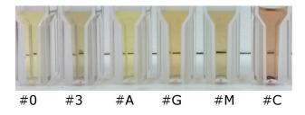
**Figure 8.** Picture of the samples: AgNP#0 (pure citrate capped silver nanoparticles); AgNP#3 (243 μM of glyphosate); AgNP#A (243 μM of AMPA); AgNP#G (243 μM of glufosinate-ammonium); AgNP#M (300 μM of glyphosate in commercial formulation 1) and AgNP#C (300 μM of glyphosate in commercial formulation 2).
