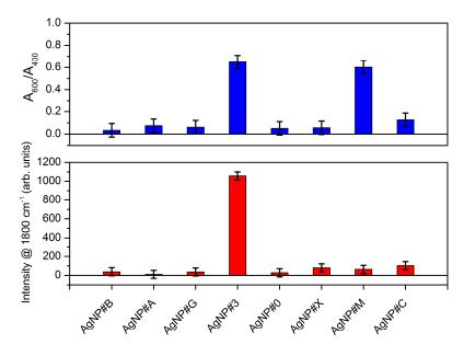
**Figure 11.** Glyphosate and interferent detection using the two transduction mechanisms. Samples: AgNP#B (tap water), AgNP#A (243 µM of AMPA), AgNP#G (243 µM of glufosinate-ammonium), AgNP#3 (243 µM of glyphosate), AgNP#0 (pure citrate-capped silver nanoparticles), AgNP#X (tap water with glyphosate at final concentration of 243 µM), AgNP#M (300 µM of glyphosate in commercial formulation 1), AgNP#C (300 µM of glyphosate in commercial formulation 2).
