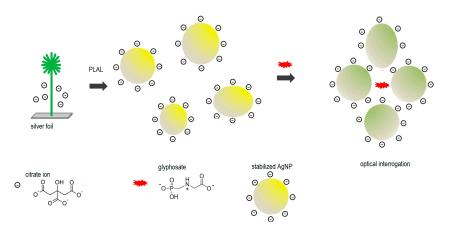
**Figure 12.** Schematic representation of the glyphosate sensing mechanism with citrate-capped colloidal AgNP.
