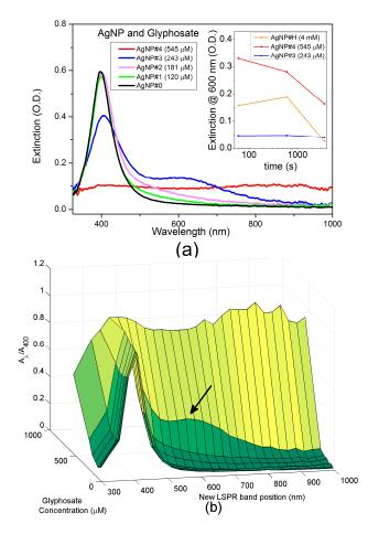
**Figure 6.** (a) UV-Vis extinction spectra of the samples with different concentrations of glyphosate. The inset shows the aggregation kinetics for three different concentrations; (b) LSPR extinction ratio as a function of the analyte concentration and the position of the new LSPR band. The arrow indicates the best response for the extinction ratio.
