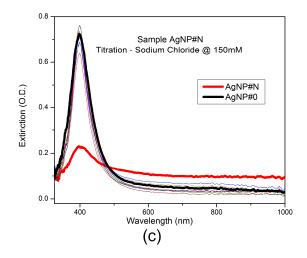
**Figure 4.** Extinction spectra of the AgNP colloidal solution (**a**) during titration with glyphosate at 40 mM (AgNP#H); (**b**) along the time for the sample with glyphosate concentration of 4 mM (AgNP#H); (**c**) during titration with sodium chloride at 150 mM (AgNP#N).
