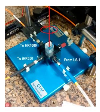
**Figure 3.** A picture of the sample holder of the experimental setup used for UV-Vis and Raman spectroscopic interrogation.
