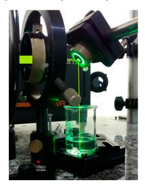
**Figure 1.** Picture of the experimental setup used for the production of the silver nanoparticles colloidal solution by Pulsed Laser Ablation in Liquid (the laser beam was highlighted).
