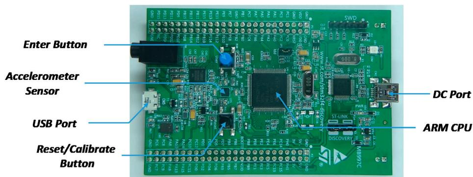
Figure 8. Data acquisition system based on the STM32F4-Discovery board.
