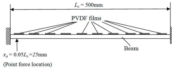
**Figure 2.** The locations of PVDF films and excitation point force on the beam.
