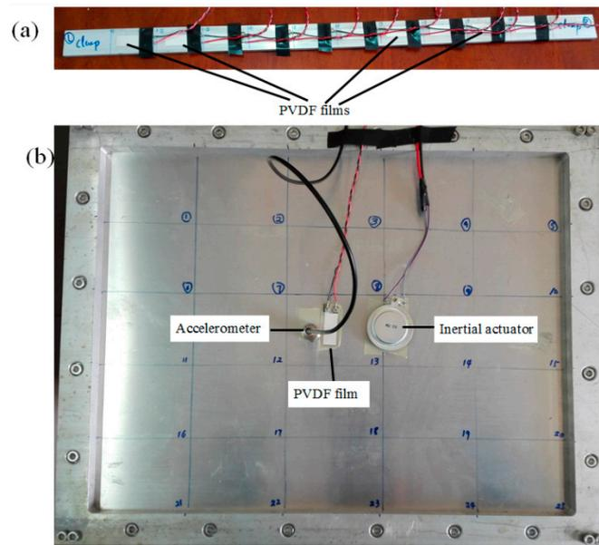
**Figure 18.** Photographs of (a) a beam bonded 10 PVDF films; (b) a clamped plate.
