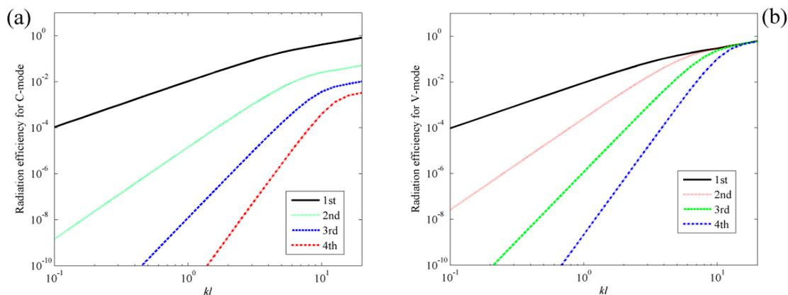
**Figure 3.** The radiation efficiencies of beam for (a) the first four C-modes; (b) the first four V-modes.
