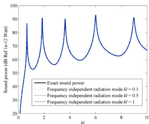
Figure 7. The sound power for beam calculated by using the first three frequency independent C-modes.
