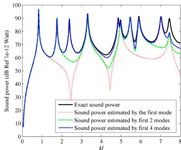
**Figure 14.** The sound power for plate calculated by using the first four frequency independent C-modes.
