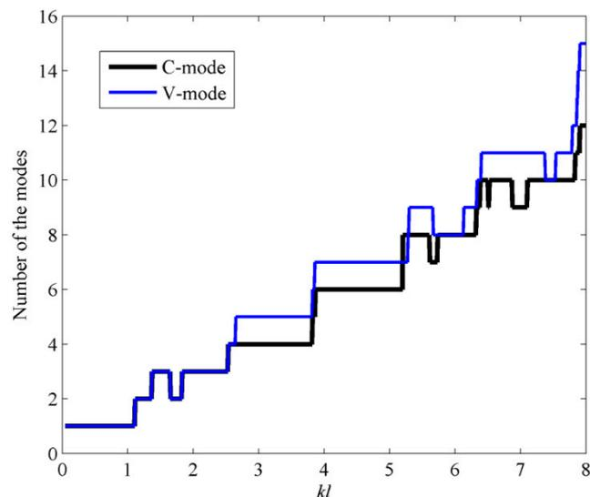
**Figure 17.** The mode number requirements by C-mode and V-mode to account for 99% of the sound power when the plate is excited by the point force.
