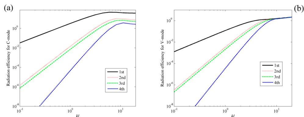
**Figure 11.** The radiation efficiencies of plate for (a) the first four C-modes; (b) the first four V-modes.
