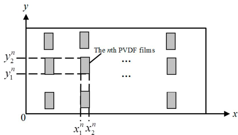
Figure 1. Rectangular PVDF films bonded on a plate.
