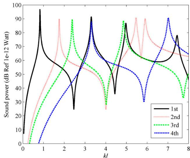
**Figure 16.** The sound power of the first four C-modes for plate under the point force excitation.
