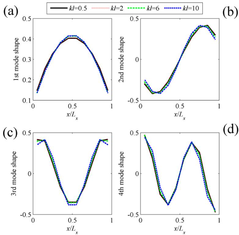
Figure 4. The shapes of (a) the first; (b) the second; (c) the third; (d) the fourth C-modes for clamped-clamped beam at different dimensionless frequencies.
