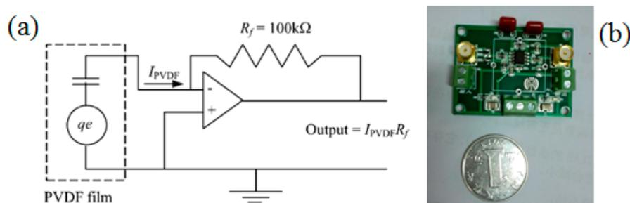
**Figure 19.** (a) Circuit schematic of a signal conditioner; (b) Photograph of the custom-built signal conditioner.
