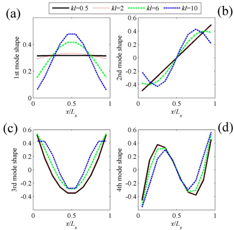
Figure 5. The shapes of (a) the first; (b) the second; (c) the third; (d) the fourth V-modes for clamped-clamped beam at different dimensionless frequencies.
