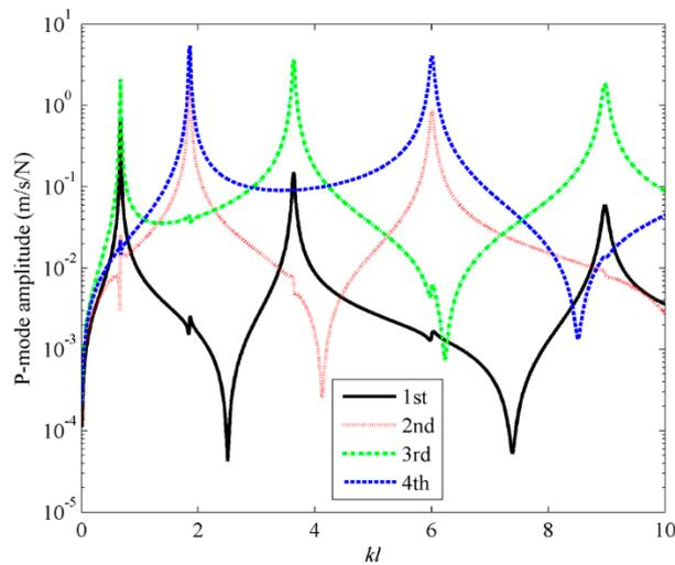
**Figure 8.** The first four C-mode amplitudes for beam under the point force excitation.
