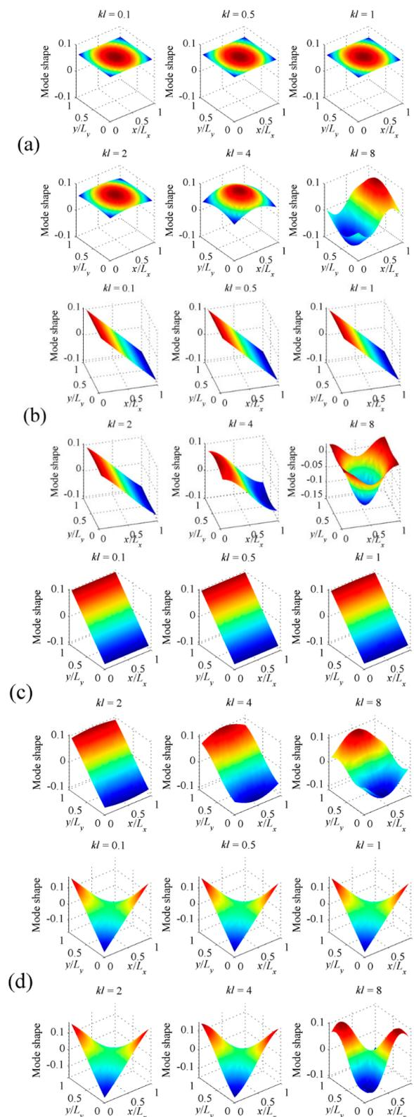
**Figure 13.** The shapes of (a) the first; (b) the second; (c) the third; (d) the fourth V-modes for clamped plate at different dimensionless frequencies.
