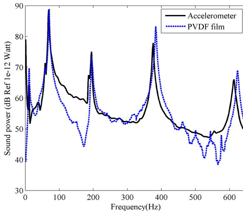
**Figure 20.** The experimental sound power for the clamped-clamped beam.
