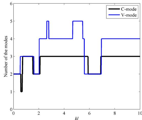
**Figure 10.** The mode number requirements by C-mode and V-mode to account for 99% of the sound power when the beam is excited by the point force.
