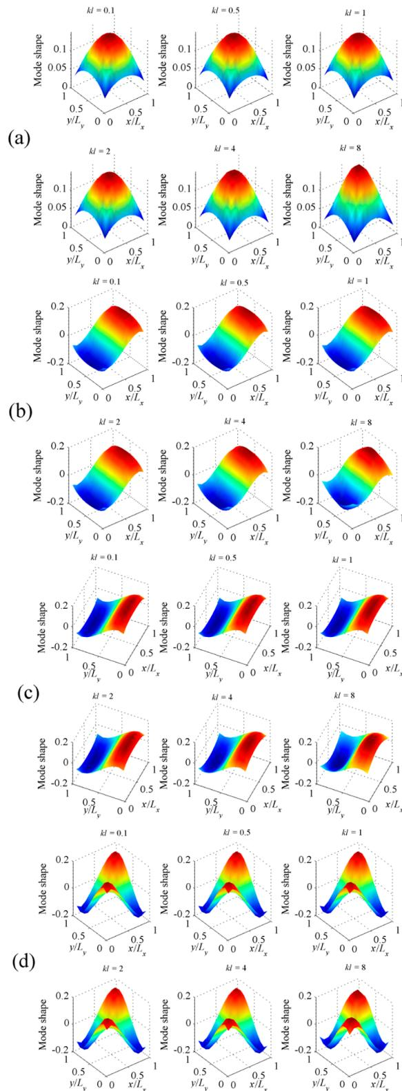
**Figure 12.** The shapes of (a) the first; (b) the second; (c) the third; (d) the fourth C-modes for clamped plate at different dimensionless frequencies.
