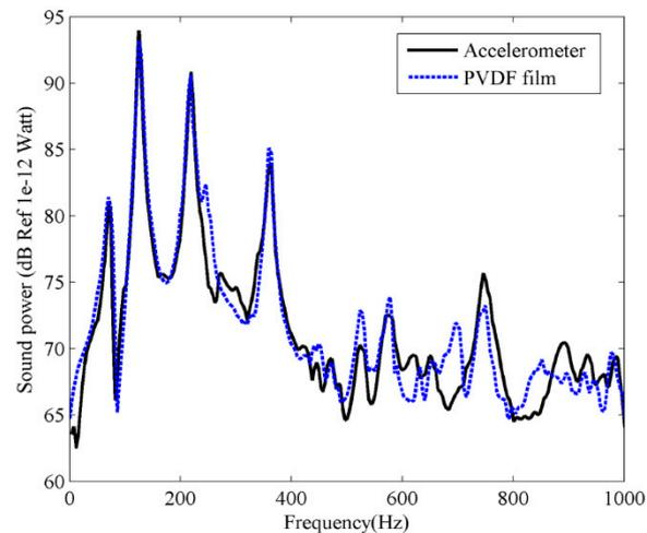
**Figure 21.** The experimental sound power for the clamped plate.
