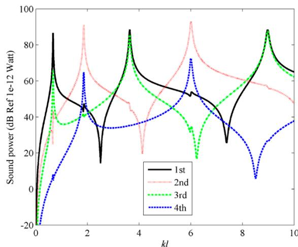
**Figure 9.** The sound power of the first four C-modes for beam under the point force excitation.
