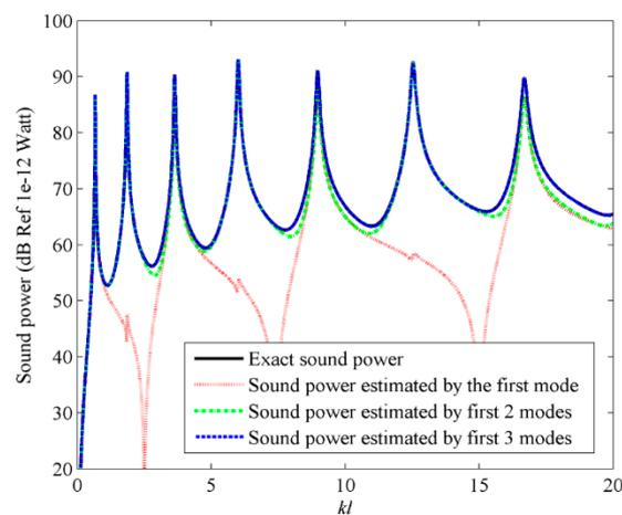
Figure 6. The sound power for beam calculated by using the frequency dependent C-modes.
