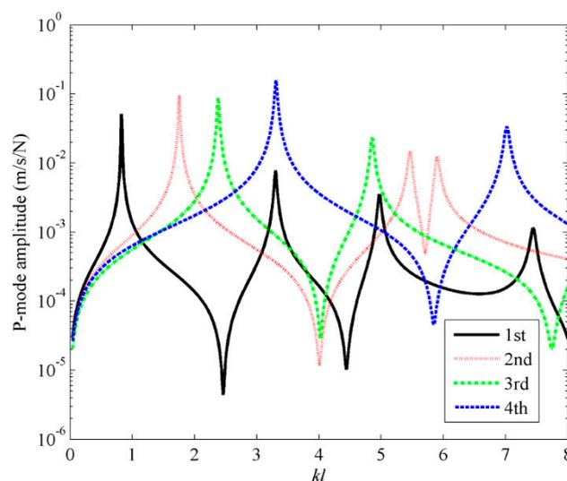
**Figure 15.** The first four C-mode amplitudes for plate under the point force excitation.
