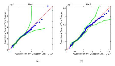
**Figure 8.** Experimental data: Q-Q plot of the search times for (a) N = 1 and (b) N = 5 versus the inverse Gaussian distribution with parameters fitted using maximum likelihood estimation. The source was placed as shown in Figure 7 and initial centroid position was fixed at [125, -125]. The green lines show 95% confidence bands [35].
