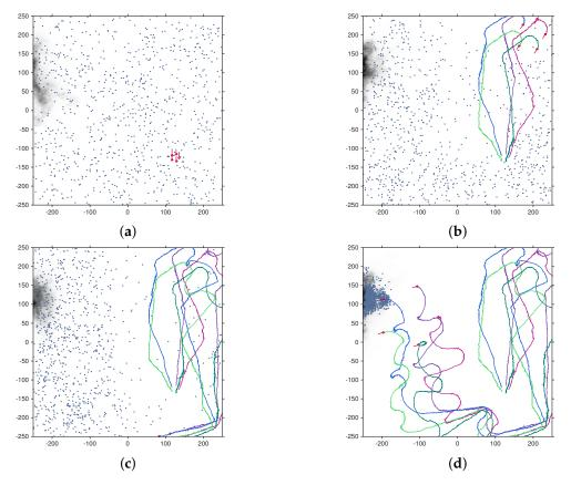
**Figure 7.** An illustrative run of the multi-robot search algorithm on the experimental dataset using N = 5 platforms. (**a**–**d**) show the positions and trajectories of the platforms at times k = 0, 10, 20 and 30, respectively. The plume from the experimental dataset can be seen in the top left of the search area, with darker areas representing higher concentrations.
