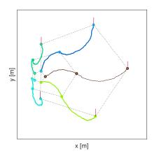
**Figure 1.** An illustration of a path of a coordinated group of N = 5 searching robots at three consecutive time instants, with the scale of the formation increasing. The small circles in the figure represent robot locations  $\mathbf{r}_k^i$ ; the vertical lines indicate the current headings  $\phi_{k}^i$ , for i = 1, ..., N.
