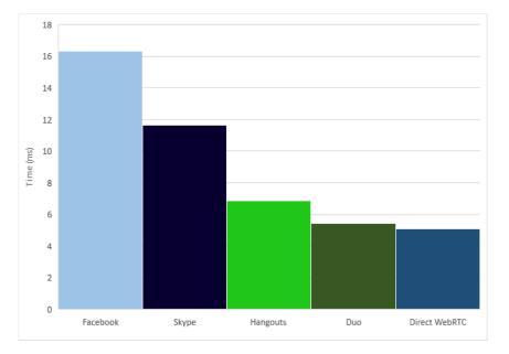
Figure 9. Average smartphone to smartphone stream delay time.
