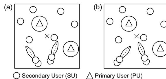
**Figure 5.** Illustration of two beamforming schemes used to evaluate the connectivity of CRAHNs: (a) randomized beamforming; (b) center-directed beamforming.
