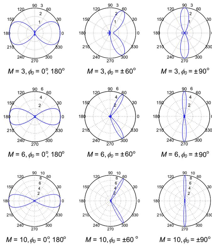
**Figure 2.** Gain patterns of ULA as the numbers of antenna elements and main beam directions are varied.
