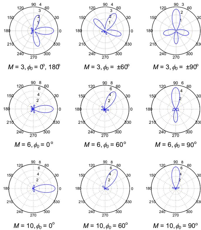
**Figure 3.** Gain patterns of UCA as the numbers of antenna elements and main beam directions are varied.
