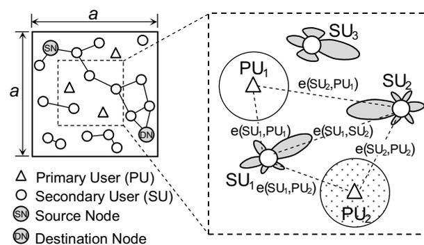
**Figure 4.** The network model of CRAHNs where SUs employ directional antennas and PUs use omnidirectional antennas.
