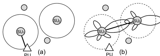
**Figure 1.** Difference in the network connectivity of CRAHNs with (a) omnidirectional antenna and (b) directional antenna.
