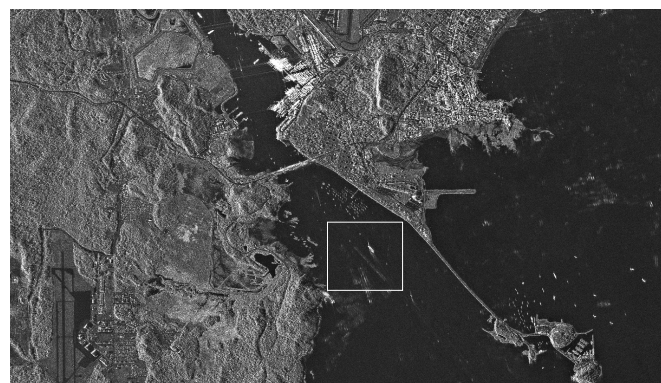
Figure 8. High-resolution, multi-look, HH polarized SAR image of the Panama Canal region acquired by the X-band TerraSAR SM mode on 31 July 2009.
