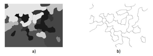
Figure 13. Example of watershed segmentation: (a) synthetic test image; and (b) the resulting segmented image.
