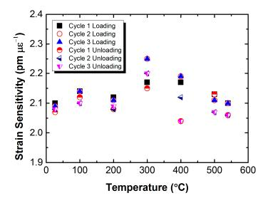
**Figure 11.** Strain sensitivity of the metal-packaged strain sensor based on the RFBG in  $H_2$ -loaded PS1250/1500 fiber obtained from mechanical load-cycling tests as a function of temperature.
