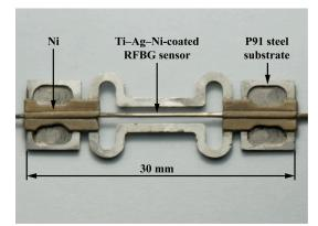
**Figure 8.** A laboratorial prototype of a metal-packaged strain sensor based on the RFBG in  $H_2$ -loaded PS1250/1500 fiber.
