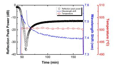
**Figure 6.** Evolution of the reflection peak power and the Bragg wavelength shift of the grating shown in Figure 1 during the isothermal annealing at 500 °C.
