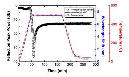
**Figure 1.** Typical evolution of the reflection peak power and the Bragg wavelength shift of one grating with the corresponding temperature profile during annealing for fabrication of the regenerated fiber Bragg grating (RFBG) in H<sub>2</sub>-loaded PS1250/1500 fiber.
