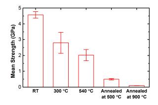
**Figure 5.** Mean tensile strengths of the bare silica optical fibers annealed at 500 °C and 900 °C respectively and tested at room temperature (26 °C), compared with those of the bare fibers without annealing tested at room temperature (26 °C), 300 °C and 540 °C [26].
