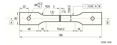
Figure 2. Pin-loaded sheet tensile test specimen with 70-mm gauge length.
