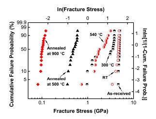
**Figure 4.** Weibull plot of the tensile strengths of the bare silica optical fibers annealed at 500 °C and 900 °C respectively and tested at room temperature (26 °C), compared with those of the bare fibers without annealing tested at room temperature (26 °C), 300 °C and 540 °C, as well as the as-received fibers tested at room temperature (26 °C) [26]. RT: room temperature
