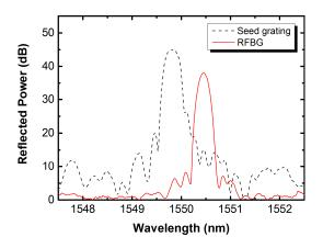
**Figure 7.** Reflection spectra of the typical type-I seed fiber Bragg grating (FBG) and its corresponding RFBG in H<sub>2</sub>-loaded PS1250/1500 fiber measured at room temperature (21 °C).
