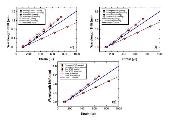
**Figure 9.** Shift in the Bragg wavelength as a function of strain obtained from tensile tests at constant temperatures of 26.5 °C (a); 100 °C (b); 200 °C (c); 300 °C (d); 400 °C (e); 500 °C (f) and 540 °C (g). FE: finite element.
