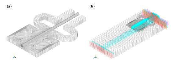
**Figure 3.** Three-dimensional (3-D) finite element (FE) model: (**a**) one half of a meshed model of a metal-packaged RFBG strain sensor, and (**b**) boundary conditions and applied load.
