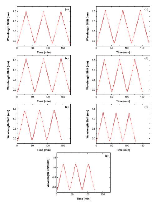
**Figure 10.** Temporal evolution of the wavelength shift during the mechanical loading cycles for the metal-packaged strain sensor based on the RFBG in H<sub>2</sub>-loaded PS1250/1500 fiber at constant temperatures of 26.5 °C (**a**); 100 °C (**b**); 200 °C (**c**); 300 °C (**d**); 400 °C (**e**); 500 °C (**f**) and 540 °C (**g**).
