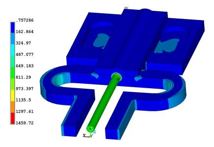
**Figure 12.** Von Mises stress distribution in the metal-packaged RFBG strain sensor at a strain of 0.26% applied to the test specimen at room temperature.
