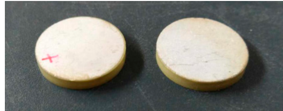
Figure 4. The positive and negative electrode surface of PZT-5 piezoelectric ceramic patches.
