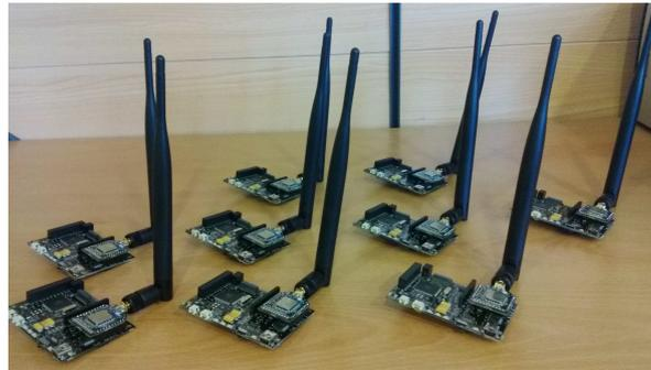
Figure 7. Waspote devices equipped with BLE module.
