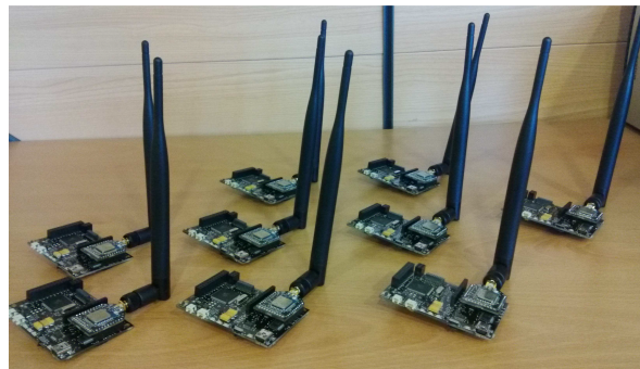
Figure 7. Wasp mote devices equipped with BLE module.
