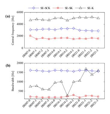
**Figure 9.** Identification results of optimal resonant frequency bands. (**a**) The optimal central frequencies; (**b**) the optimal bandwidth.
