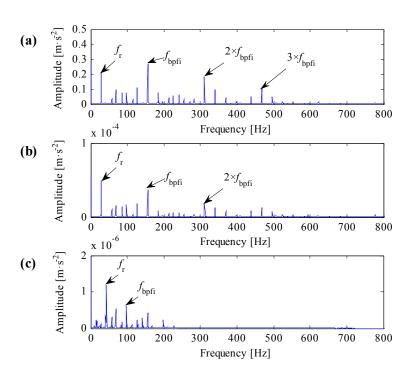
**Figure 11.** Analysis results of data IR021-3. (**a**) The result based on the improved correlated kurtosis; (**b**) the result based on the kurtosis of squared envelope signal; (**c**) the result based on the spectral kurtosis of squared envelope signal.
