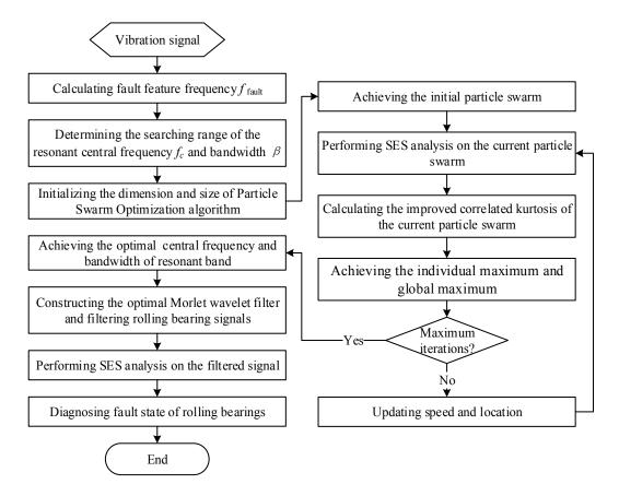
Figure 3. Flowchart of the proposed optimal resonant band demodulation method.
