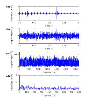
**Figure 4.** (a) Repetitive transient impulses and impulsive noises in the simulation signal; (b) the simulation signal with white Gaussian noise; (c) the spectrum of the simulation signal; (d) the SES of the simulation signal.
