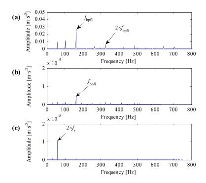
**Figure 10.** Analysis results of data IR007-0. (**a**) The result based on the improved correlated kurtosis; (**b**) the result based on the kurtosis of squared envelope signal; (**c**) the result based on the spectral kurtosis of squared envelope signal.
