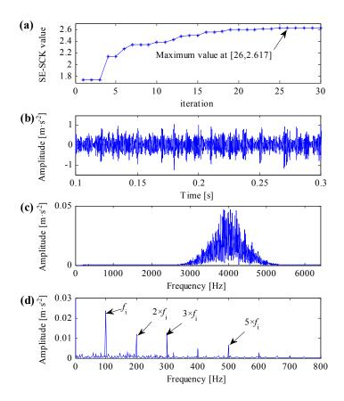
**Figure 5.** Analysis results of the proposed optimal resonant band demodulation based on the improved correlated kurtosis. (**a**) The iterative computation results of the PSO; (**b**) the filtered signal by optimal Morlet wavelet filter; (**c**) the spectrum of the filtered signal; (**d**) the SES of the filtered signal.
