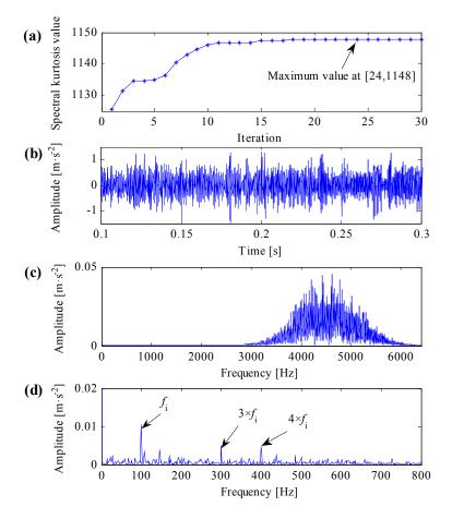
**Figure 7.** Analysis results of optimal resonant band demodulation based on spectral kurtosis of the squared envelope signal. (a) The iterative computation results of the PSO; (b) the filtered signal by optimal Morlet wavelet filter; (c) the spectrum of the filtered signal; (d) the SES of the filtered signal.
