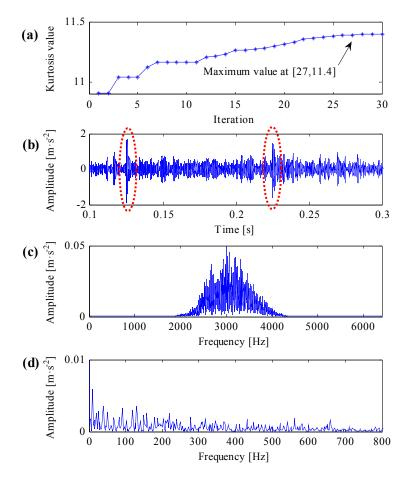
**Figure 6.** Analysis results of optimal resonant band demodulation based on kurtosis of the squared envelope signal. (**a**) The iterative computation results of the PSO; (**b**) the filtered signal by optimal Morlet wavelet filter; (**c**) the spectrum of the filtered signal; (**d**) the SES of the filtered signal.
