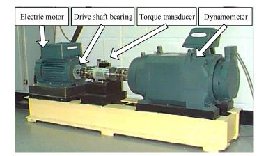
Figure 8. The bearing test rig of the CWRU Bearing Data Center [27].
