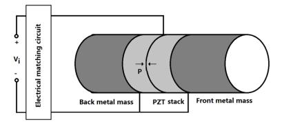
Figure 2. A high power sandwiched piezoelectric transducer with matching circuit.
