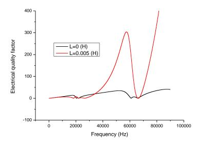
Figure 6. Frequency response of the electric quality factor.
