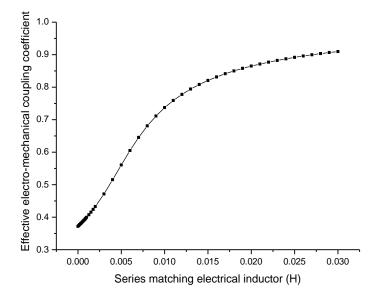
**Figure 9.** Dependency of the effective electromechanical coupling coefficient on the series matching inductor.
