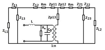
**Figure 4.** Electro-mechanical equivalent circuit of a sandwiched piezoelectric transducer with a series matching inductor.
