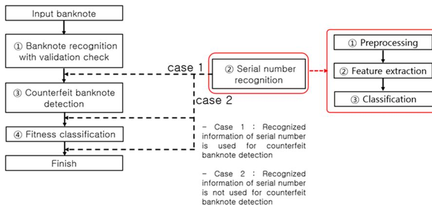
**Figure 17.** Serial number recognition process flow.
