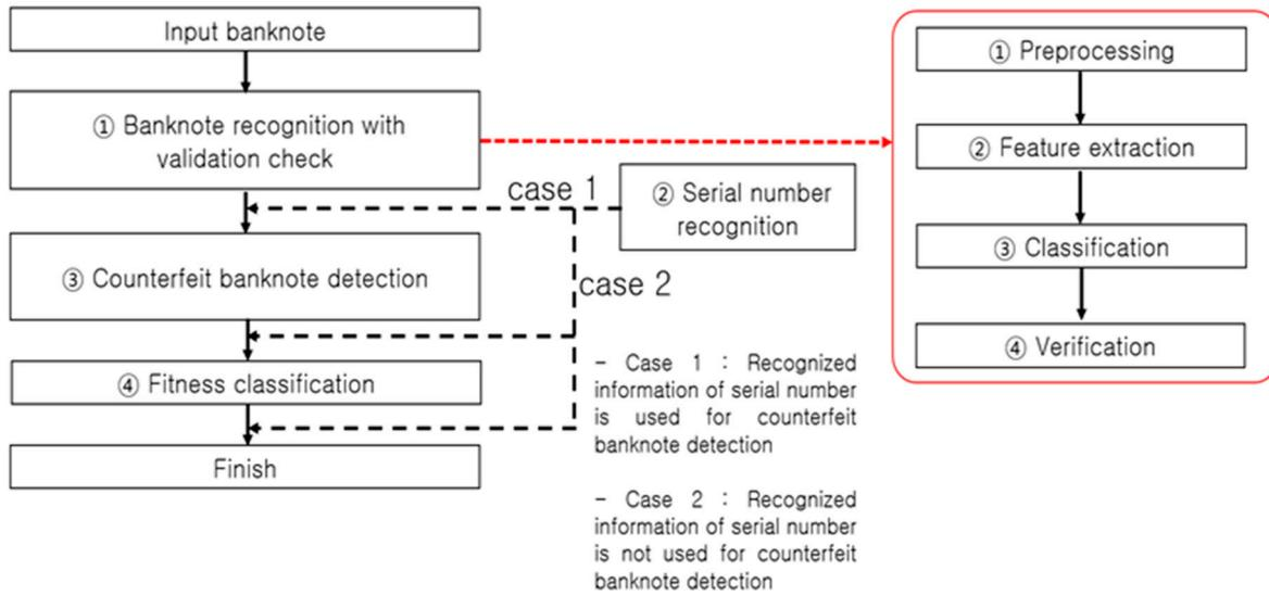
Figure 5. Banknote recognition process flow.
