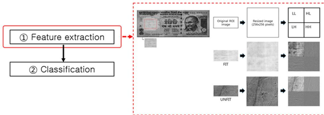
**Figure 22.** Feature extraction in the fitness classification process flow.
