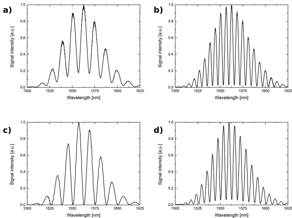
**Figure 7.** The measurement signal for the 1550 nm source. The Fabry-Pérot interferometer made by: optical fiber and cavity length: (a) 100  $\mu\text{m}$ ; (b) 200  $\mu\text{m}$ ; optical fiber with  $\text{TiO}_2$  thin film and cavity length: (c) 100  $\mu\text{m}$ ; (d) 200  $\mu\text{m}$ .
