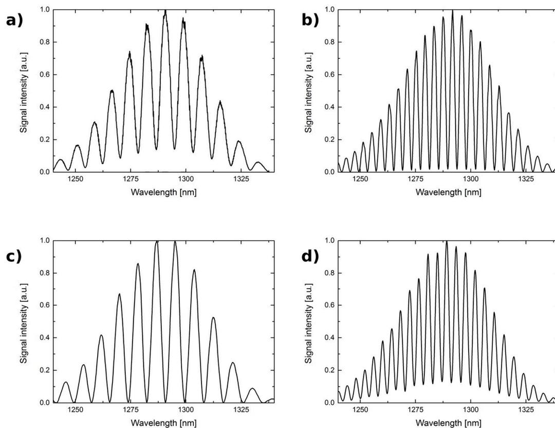
**Figure 6.** The measurement signal for the 1290 nm source. The Fabry-Pérot interferometer made by: optical fiber and cavity length: (a)  $100 \mu\text{m}$ ; (b)  $200 \mu\text{m}$ ; optical fiber with  $\text{TiO}_2$  thin film and cavity length: (c)  $100 \mu\text{m}$ ; (d)  $200 \mu\text{m}$ .
