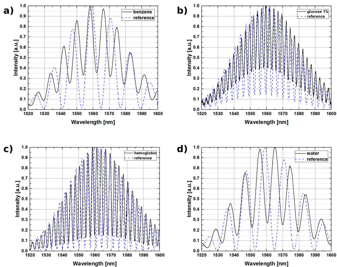
**Figure 8.** Measurements of Fabry-Pérot interferometer carried out with an optical fiber coated with  $\text{TiO}_2$  layer when the cavity is filled with: (a) benzene; (b) glucose (1% solution); (c) hemoglobin (13.4 g/dL); and (d) water.
