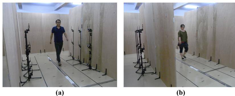
**Figure 3.** Experimental setup for walker classification in: (a) LOS scenario; (b) NLOS scenario.
