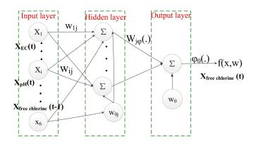
Figure 4. BP (Back Propagation) neural network structure of free chlorine.
