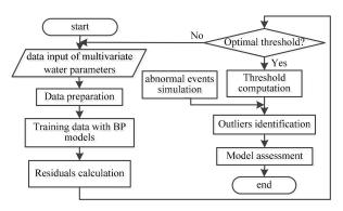
Figure 2. Procedure in the off-line phase.
