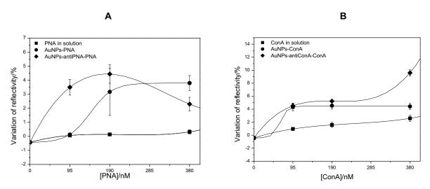
**Figure 5.** Mean value and standard deviation of the variation of reflectivity on spots of antibody anti-PNA (**A**) and antibody anti-ConA (**B**) after injection of free PNA (**A**) and ConA (**B**) in solution, covalently linked to gold NPs and captured by gold NPs functionalized with anti-PNA or anti-ConA.
