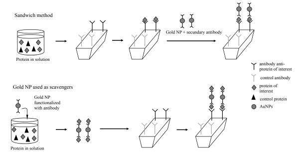
**Figure 1.** Comparative representation of the application of gold NPs in the sandwich method, where the proteins in solution are directly injected on the biosensor, and the application of gold NPs as protein scavengers, where the NPs are firstly mixed with the proteins in solution and then injected on the biosensor.
