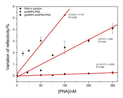
**Figure 6.** Average values and standard deviation of the variation of reflectivity as a function of the concentration of PNA detected by SPR. Linear fitting was applied for each method (red line). The linear equation and the correlation coefficient calculated for each method are displayed beside the correspondent data.
