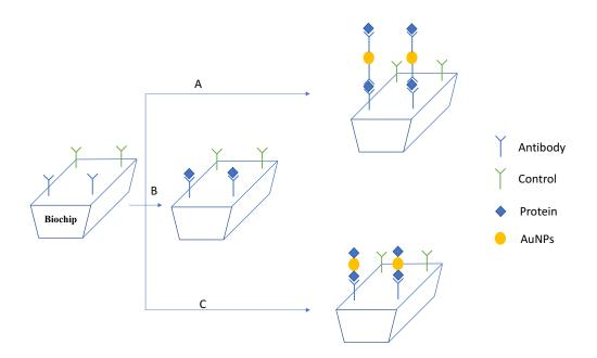
**Figure 2.** Representation of the SPR assays: Firstly, the biosensor was functionalized with antibody anti-ConA and anti-PNA. Following, (**A**) protein captured by AuNPs functionalized with antibody anti-ConA or anti-PNA, (**B**) protein in solution or (**C**) protein covalently linked to AuNPs was injected on the biosensor.
