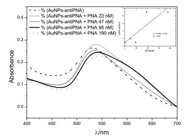
**Figure 7.** UV-Vis spectra of gold NPs functionalized with antibody anti-PNA after incubation with PNA solution at different concentrations. Insert: Linear fitting of LSPR shift of gold NPs functionalized with antibody anti-PNA as a function of the concentration of PNA in solution.
