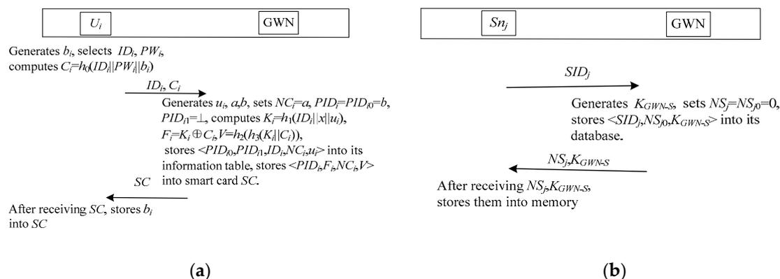
Figure 4. The registration phase. (a) The user registration phase; (b) The sensor node registration phase.
