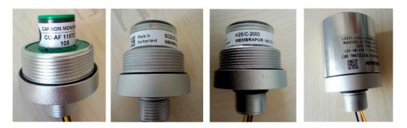
Figure 3. Electrochemical sensors.
