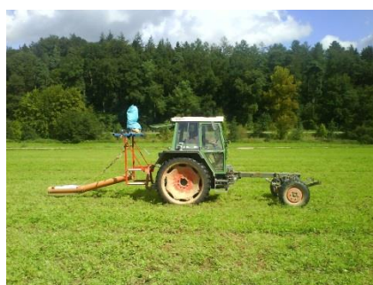
Figure 2. Mounting of the EM38 on a metal-free sledge pulled by a tractor (constructed after Corwin and Lesch [7]).
