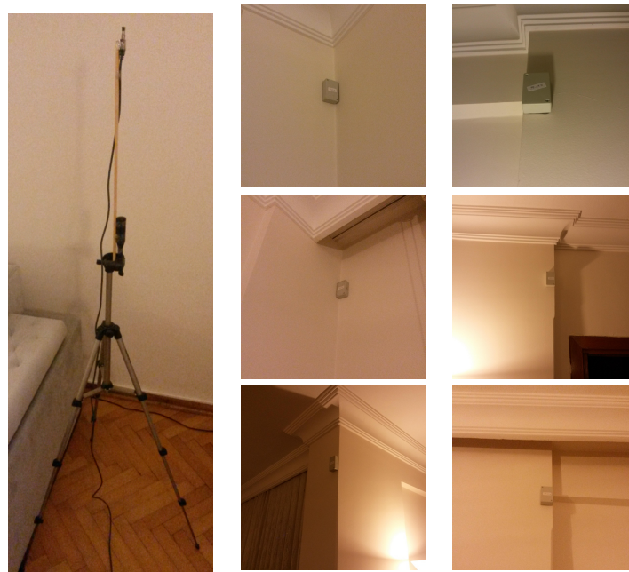
Figure 10. Bluetooth dongle on a tripod and beacons mounted on the walls.
