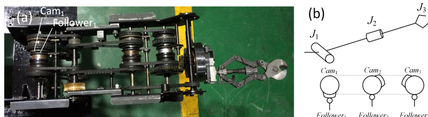
Figure 12. (a) shows the general structure of the manipulator, and (b) shows the illustration of the cam switch method for manipulator joints. J_1 represents the shoulder joint; J_2 represents the wrist joint; and J_3 represents the scissors.
