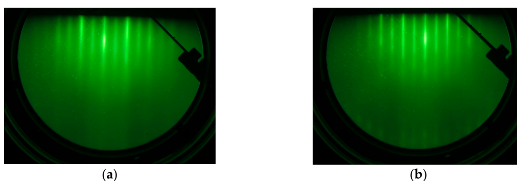
Figure 2. Reflection high-energy electron diffraction (RHEED) images of the \text{GaO}_x layer grown on the (a) MgO underlying layer and (b) Fe bottom electrode after an in-situ annealing ((110) azimuth of MgO substrate).
