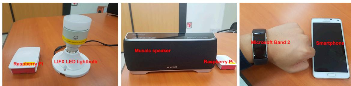
**Figure 19.** LIFX LED lightbulb (left), Musaïc streaming speaker (middle), and Microsoft Band 2 (right).
