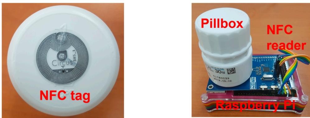
**Figure 16.** The pillbox with an NFC tag (left) and pillbox holder (right) consisting of a Raspberry Pi and NFC reader.
