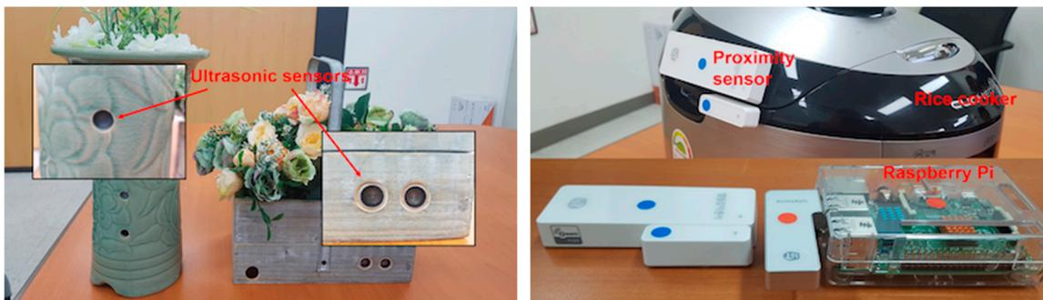
Figure 18. Ultrasonic sensors (left) and rice cooker embedded with proximity sensors (right).
