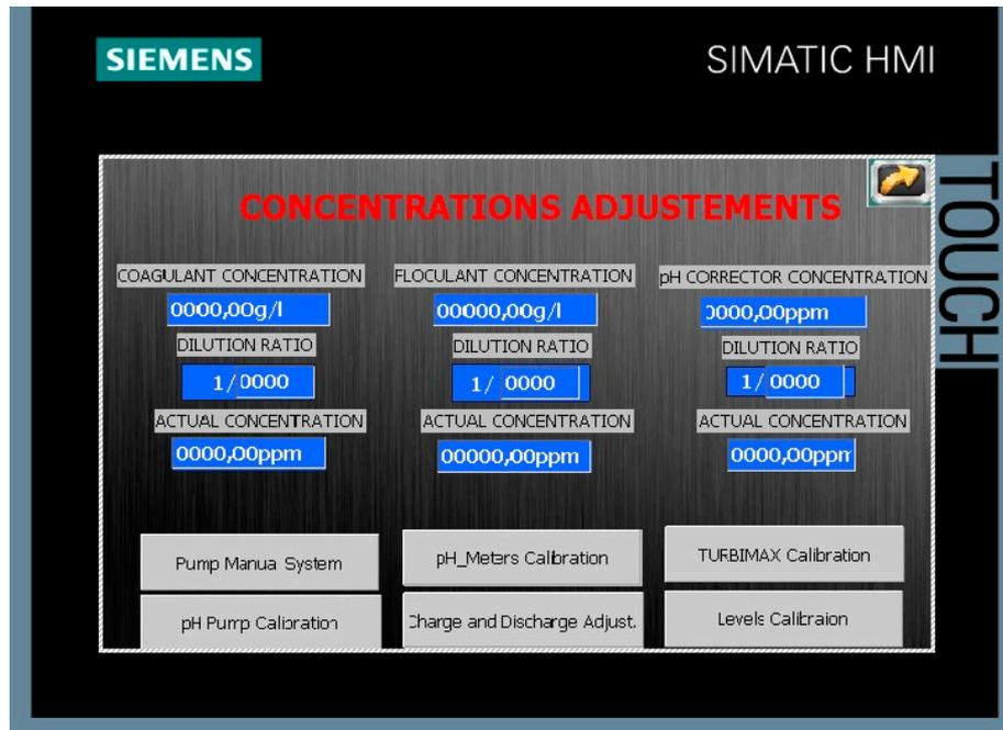
Figure 7. Screen to modify concentrations in the HMI.
