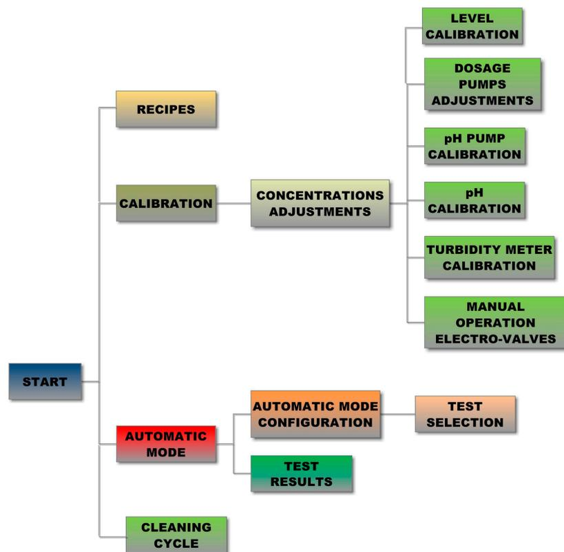
Figure 6. Navigation tree of the HMI.
