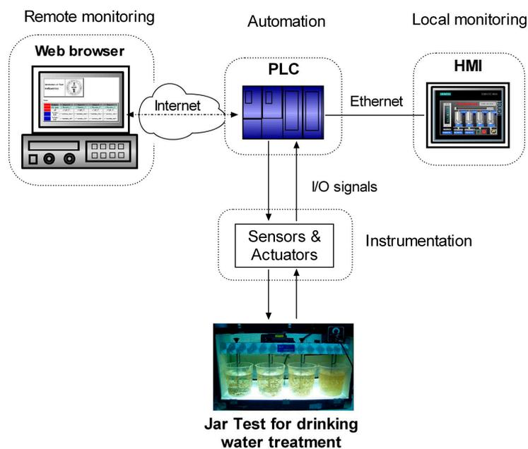
**Figure 2.** Block diagram of the developed system to automate and monitor the JT.
