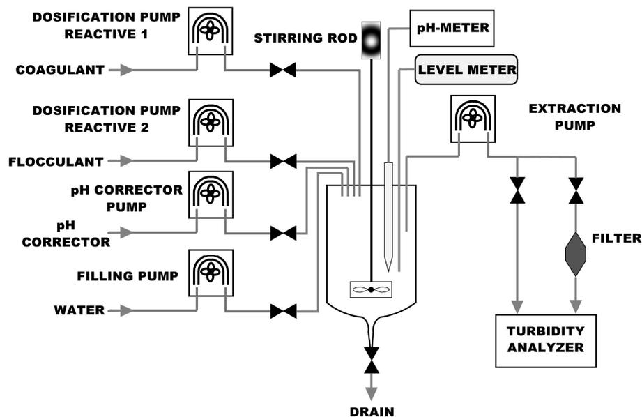
Figure 5. Fluidic diagram of the proposed solution including the sensors and actuators.
