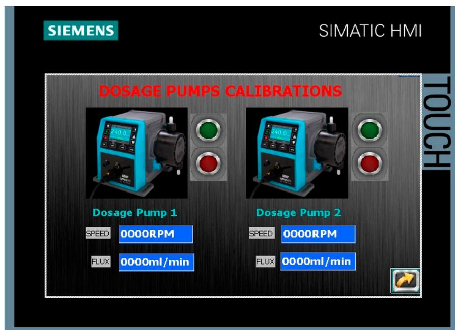
Figure 8. Screen to calibrate the dosage pumps in the HMI.
