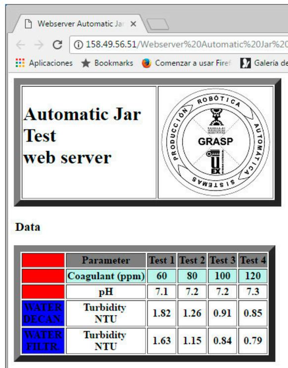
Figure 15. Web page for remote monitoring of the JT results.
