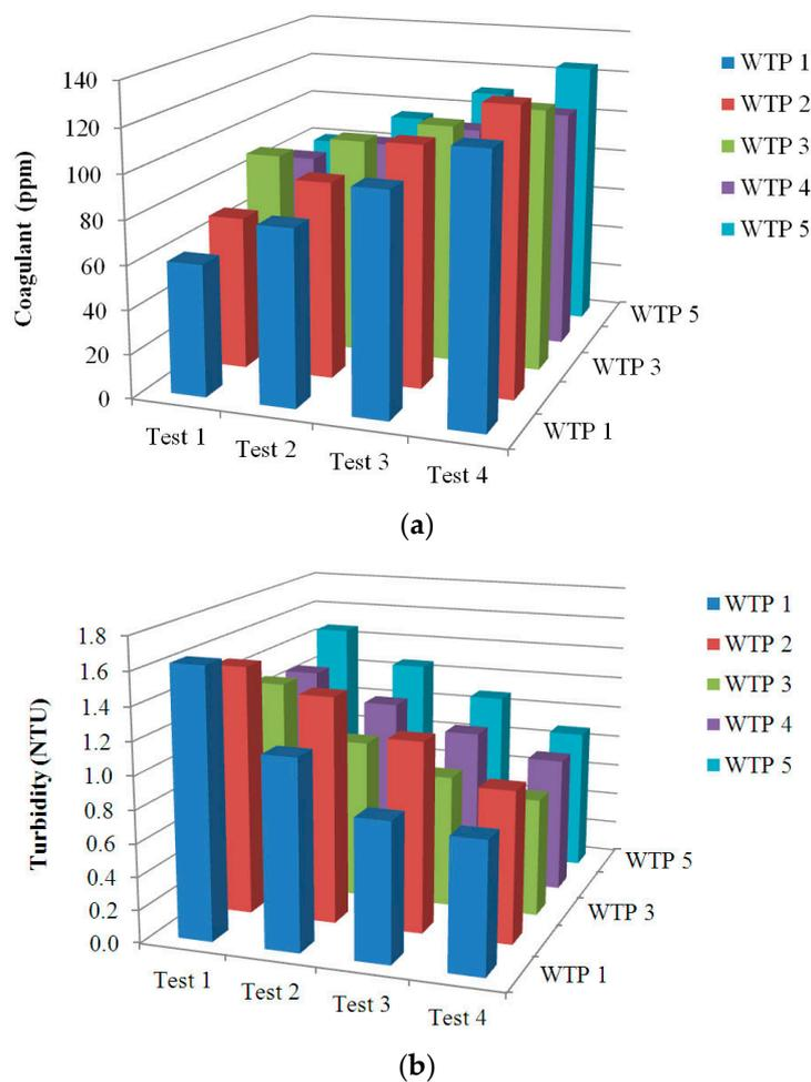
**Figure 12.** Three-dimensional graph of results of analyses performed: (a) Coagulant dosage; (b) Turbidity of filtered water.
