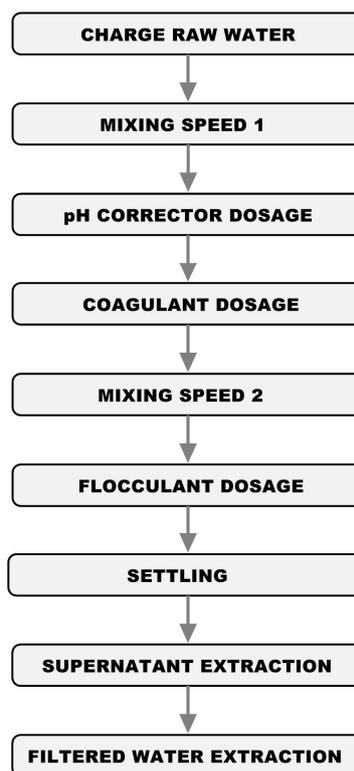
Figure 1. Flowchart of the JT procedure.
