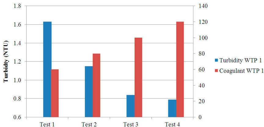
Figure 13. Turbidity and coagulant dosage values for each vessel in the JT of the WTP 1.
