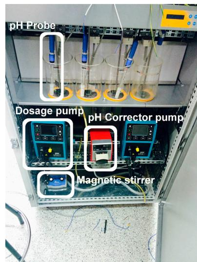
Figure 10. Front view of the prototype.
