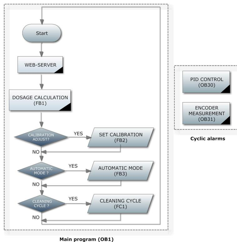
**Figure 3.** Flowchart of the program of the PLC.
