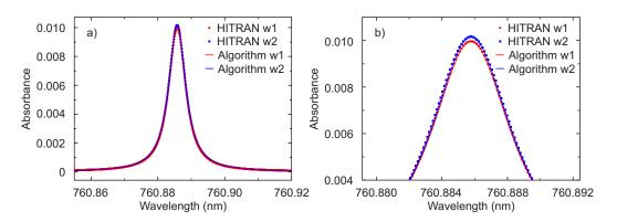
**Figure 9.** (a) comparison of the absorbance of the R7Q8 line extracted with the algorithm (solid lines; Algorithm w1, Algorithm w2) and the expected lines from HITRAN database (points; HITRAN w1, HITRAN w2) for the window 1 (w1, d = 11 mm) and window 2 (w2, d = 4 mm); (b) enlargement of the peak maximum for the same data.
