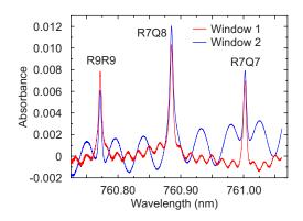
**Figure 8.** Typical absorbance for the three lines R9R9 (760.77 nm), R7Q8 (760.89 nm) and R7R7 (761.003 nm) of the  $O_2$  near infrared A-band. Superimposed to the absorption features are the interferences caused by the window 1 (d = 11 mm) and window 2 (d = 4 mm). The measurement is taken at atmospheric conditions.
