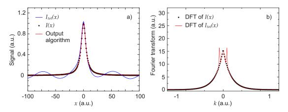
**Figure 4.** First scenario: disturbance with an FSR comparable to the line width. (a) simulated experimental total signal  $I_{tot}(x)$  (blue line), Lorentzian line shape signal I(x) (black dots) and extracted signal obtained with the algorithm (red line); (b) DFT of the total signal  $|F(I_{tot}(x))(k)|$  (red line) and DFT of the Lorentzian signal |F(I(x))(k)| (black points).
