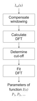
**Figure 1.** Schematic flow diagram of the steps of the algorithm to extract a signal I(x) from a total signal  $I_{tot}(x)$ .
