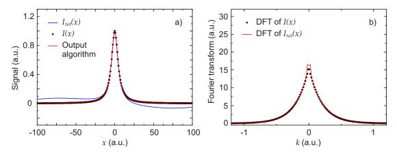
**Figure 5.** Second scenario: weak disturbance with an FSR as large as the measuring window. (a) simulated experimental total signal  $I_{tot}(x)$  (blue line), Lorentzian line shape signal I(x) (black dots) and extracted signal obtained with the algorithm (red line); (b) DFT of the total signal  $|F(I_{tot}(x))(k)|$  (red line) and DFT of the Lorentzian signal |F(I(x))(k)| (black points).
