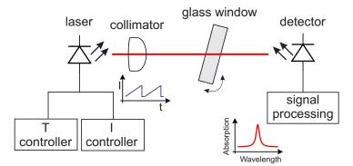
Figure 7. Schematic diagram of the setup used for the absorption spectroscopy experiments.
