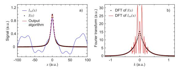
**Figure 6.** Third scenario: strong multiple disturbances. (a) simulated experimental total signal  $I_{tot}(x)$  (blue line), Lorentzian line shape signal I(x) (black dots) and extracted signal obtained with the algorithm (red line); (b) DFT of the total signal  $|F(I_{tot}(x))(k)|$  (red line) and DFT of the Lorentzian signal |F(I(x))(k)| (black points).
