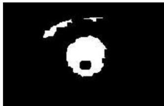
Figure 4. Detection of the infrared reflection in the pupil.
