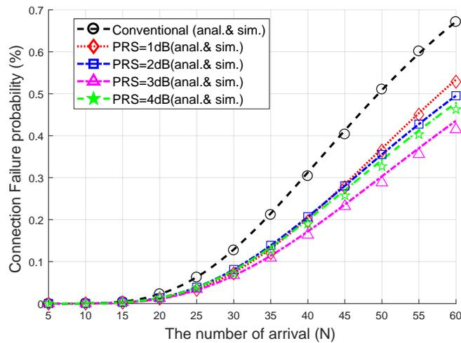
Figure 9. Connection failure probability ( $N_{max} = 8$ ,  $V = 20$ ).
