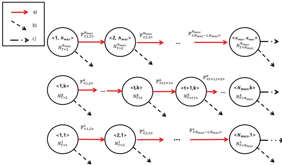
**Figure 2.** Markov chain model of the devices. State  $\langle t, k \rangle$  indicates that the devices with the trial number  $T_u = t$  and  $Z_u = k$ . Note that state transitions occur when (a) random access (RA) failure, (b) RA success, and (c) connection failure occurs, respectively.
