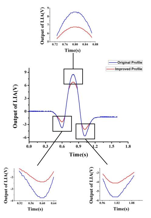
**Figure 4.** Original profile of the second harmonic (blue line) and the improved profile with modulation index adjustment (red line). Softer inflection points are shown in detail.
