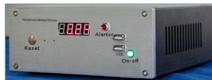
**Figure 2.** The photograph of this PA methane sensor.
