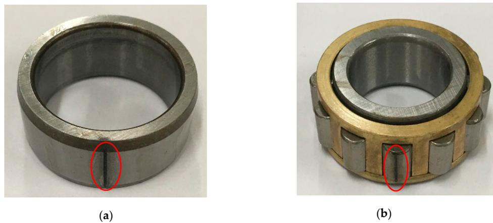
**Figure 8.** (a) Inner-race fault (b) rolling-element fault.
