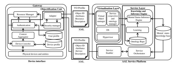
**Figure 4.** Functional modules of a web of object-based AAL platform especially in a mental healthcare scenario.
