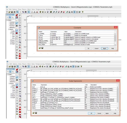
Figure A3. COMSOL constants and expressions for calculating magnetic force and velocity.
