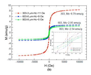
**Figure A1.** Magnetization curves for (a) M-270 streptavidin beads and (b) COMPEL<sup>TM</sup> beads. (Reprinted with permission from refs. [56]—Copyright 2005 Elsevier, and [57]—Copyright Bangs Laboratories, Inc.<sup>TM</sup>).
