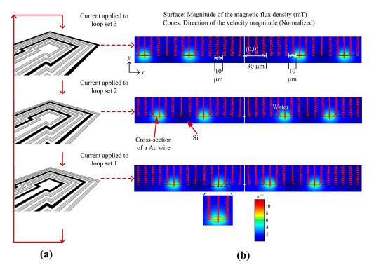
**Figure 1.** (a) Design of the magnetic actuator; (b) Magnitude of magnetic flux density (surface plot) when 125 mA of electric current was applied sequentially to the 3 loop sets.
