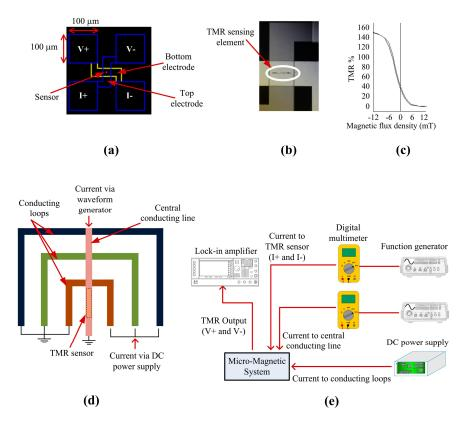
**Figure 3.** (a) Design of the TMR sensor; (b) Fabricated TMR sensing element; (c) Sensitivity of the TMR sensor; (d) MA and TMR sensor integration; (e) Experimental setup for magnetic bead detection.
