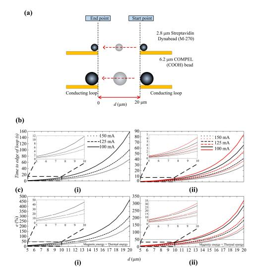
**Figure 4.** (a) Travel path of the SPBs; (b) The time taken for (i) COMPEL<sup>™</sup> bead and (ii) Dynabead<sup>®</sup> (black lines) and polystyrene YG particle tagged with a Dynabead<sup>®</sup> (red lines) to travel to the edge of a loop, from a maximum distance of 20 µm from the edge; (c) Error caused by diffusion for (i) COMPEL<sup>™</sup> bead and (ii) Dynabead<sup>®</sup> and polystyrene YG particle tagged with a Dynabead<sup>®</sup>.
