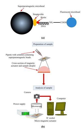
**Figure A2.** (a) Attachment of DNA to a superparamagnetic bead; (b) Experimental setup for manipulation of magnetic beads by the magnetic actuator.
