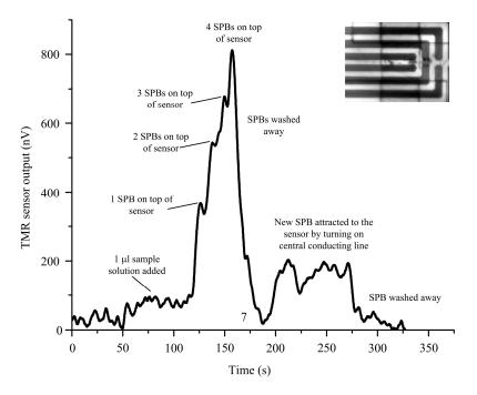
Figure 7. Manipulation and detection of magnetic beads by the micro-chip.
