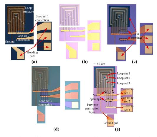
**Figure 2.** Fabrication of the micro-magnetic actuator. (a) Gold wires after deposition and patterning; (b) Parylene passivation layer on top of gold wires; (c) Vias and pads opened by oxygen plasma etching; (d) Patterned photoresist layer to connect the loop structures to bonding pads; (e) Final fabricated device.
