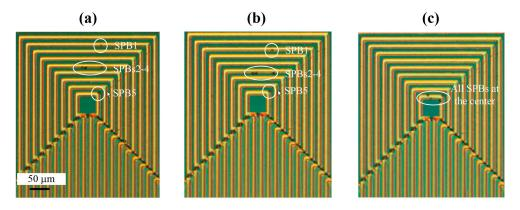
**Figure 5.** Experiments demonstrating the manipulation and transportation of COMPEL<sup>TM</sup> beads utilizing the magnetic actuator. (a) Five magnetic beads on the MA; (b) Movement of magnetic beads towards the center of the MA; (c) All magnetic beads manipulated to the center of the MA.
