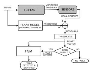
**Figure 1.** Schematic of the classical model-based FDI strategy for FC plants based on parity equations with output errors [12], residual binarization, and FSM.
