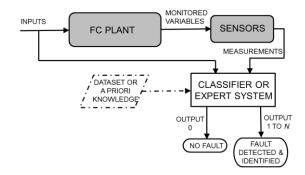
Figure 2. Schematic of the data-driven FDI strategy applied to FC plants.
