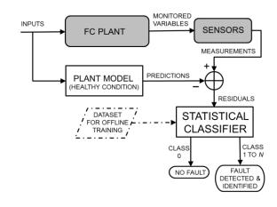
**Figure 3.** Schematic of the hybrid FDI strategy for FC plants, where residuals generated by the parity equations are processed by an adequately trained statistical classifier.
