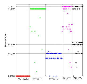
**Figure 6.** Binary vectors, from  $[0\ 0\ 0\ 0]$  to  $[1\ 1\ 1\ 1\ 1]$ , produced by the model-based FDI system (see Figure 1) for the SOFC plant operating under healthy and faulty conditions. For a given fault, each asterisk indicates the binary vector produced by a given combination between the operating condition and fault size. The constant-voltage control for the SOFC plant is considered, the maximum percentage error is 4%, and the relative threshold  $\Omega$  is 4.5%.
