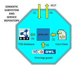
Figure 15. Semantic Subsystem and Service Repository Registration diagram.
