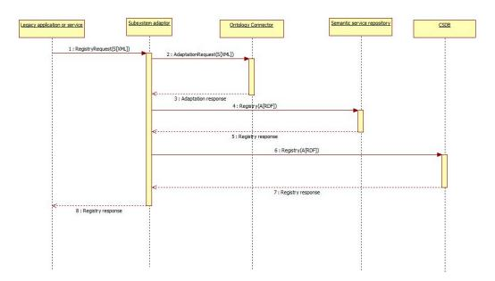
Figure 12. Service registration sequence diagram.
