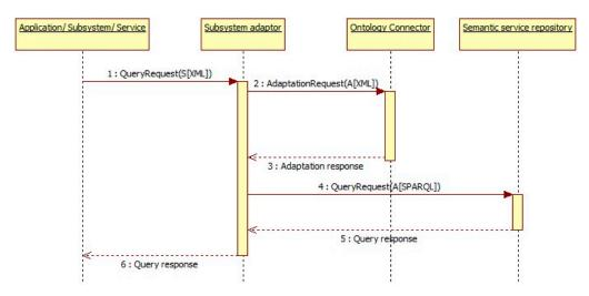
Figure 13. Discovery sequence diagram.
