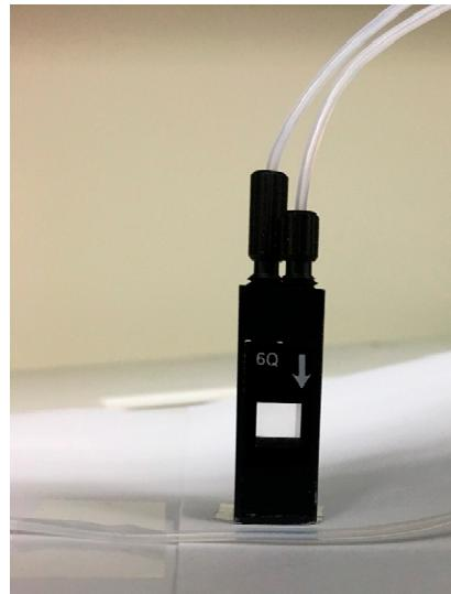
**Figure S5.** The commercial flow-cuvette connected to the tubing of the flow system. During the measurements the cuvette was placed inside the spectrophotometer.
