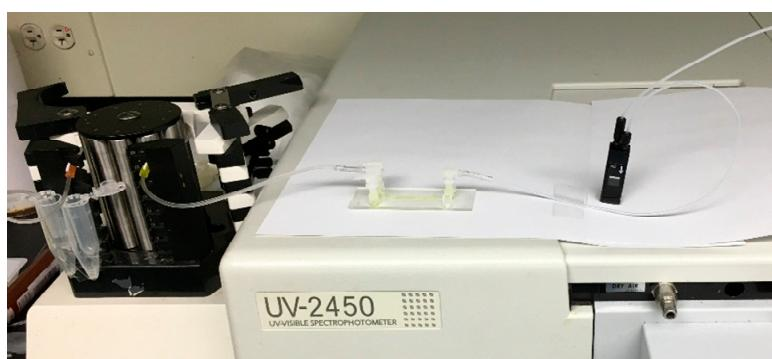
**Figure S4.** A different view of the experimental setup that was used to analyze the signal transduction process. The flow of solution was controlled by a Gilson MINIPULS® 3, which was used to push solution through the enzymatic flow cell and then into the flow-through cuvette before being discharged into a waste beaker. In this illustration, the flow through cuvette has been plumbed into the system, to illustrate the process.
