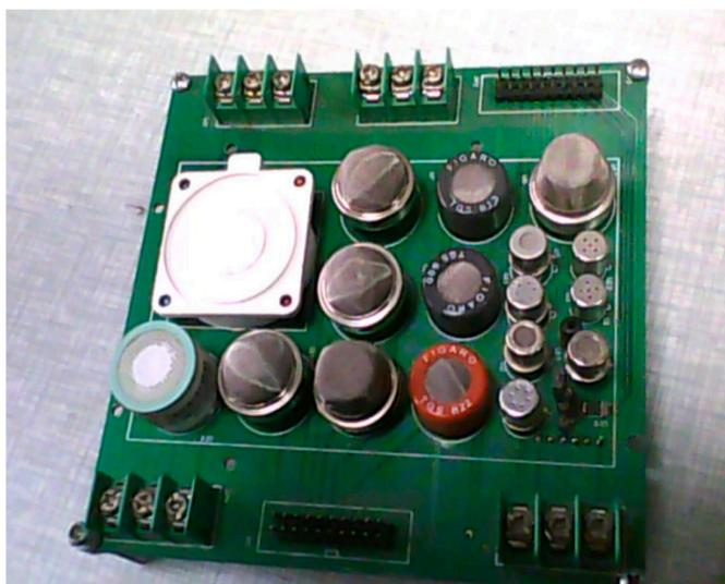
**Figure 1.** Electronic nose sensor array.
