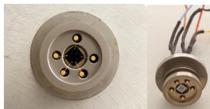
**Figure 6.** The pressure-sensitive chip modular package.
