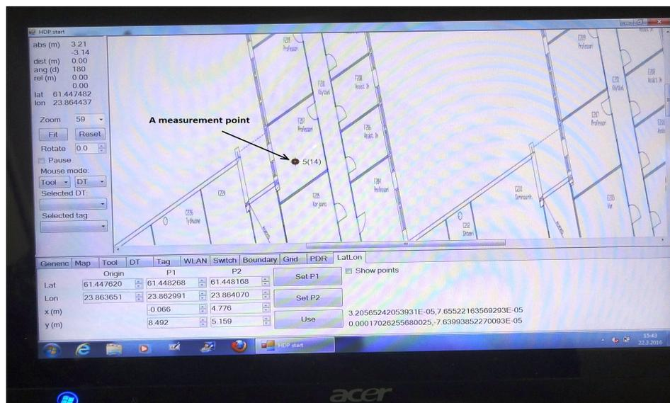
**Figure 2.** The Acer windows tablet used for collecting data with a sample measurement point shown here. The number outside the parentheses (here, 5) is the fingerprint index, and the number inside (here, 14) shows the number of access points heard in this point.
