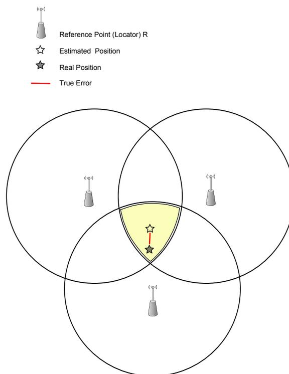
**Figure 1.** Positioning using reference points.
