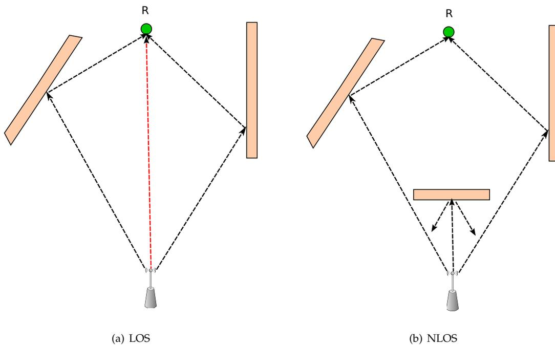
**Figure 2.** (a) Line-of-sight (LOS) vs. (b) non-line-of-sight (NLOS).
