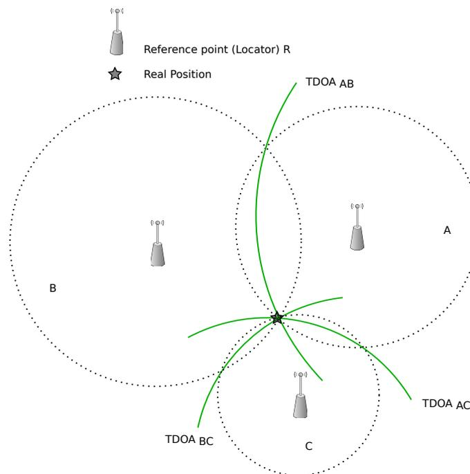
**Figure 6.** Time difference of arrival (TDoA)-based algorithms.
