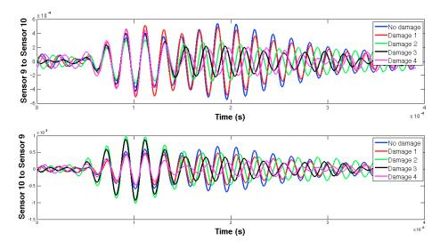
Figure 27. EMPD at 50 kHz. Tone-burst sent and measured between sensors 9 and 10.
