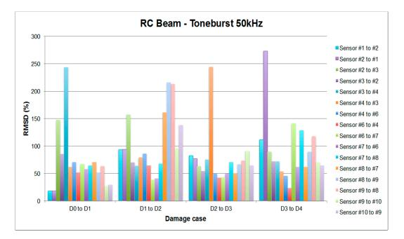
Figure 29. RMSD values for the RC beam.
