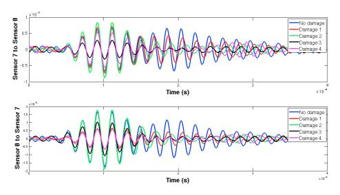
Figure 25. EMPD at 50 kHz. Tone-burst sent and measured between sensors 7 and 8.
