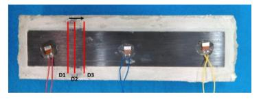
Figure 11. Damage scenario for an FRP-strengthened concrete specimen (I).
