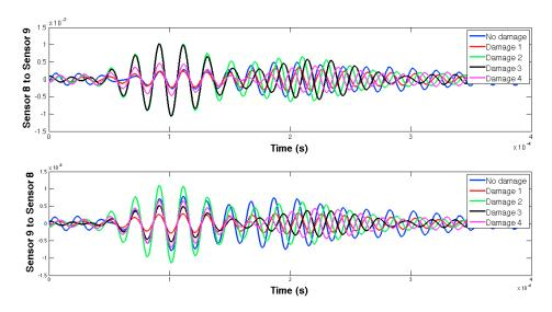
Figure 26. EMPD at 50 kHz. Tone-burst sent and measured between sensors 8 and 9.
