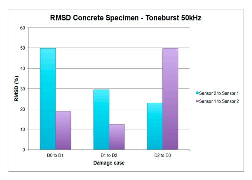
Figure 16. RMSD values for the concrete specimen.
