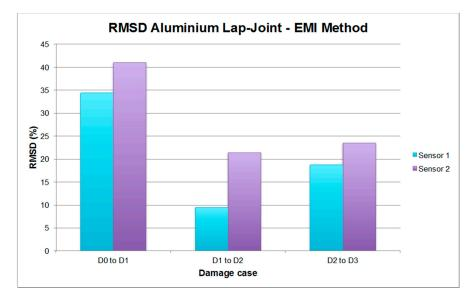
Figure 9. RMDS values for the bolt-jointed aluminium beam corresponding to the EMI method.
