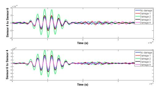
Figure 23. EMPD at 50 kHz. Tone-burst sent and measured between sensors 4 and 6.
