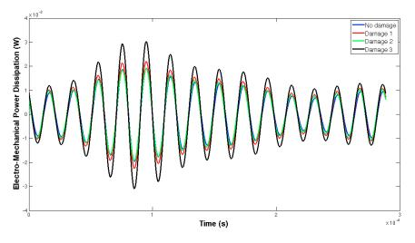
Figure 13. EMPD at 50 kHz. Tone-burst sent from sensor 1 to sensor 2.
