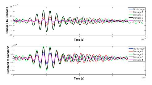
Figure 21. EMPD at 50 kHz. Tone-burst sent and measured between sensors 2 and 3.
