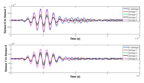
Figure 24. EMPD at 50 kHz. Tone-burst sent and measured between sensors 6 and 7.
