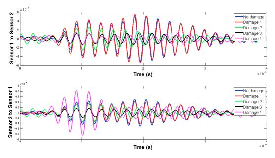
Figure 20. EMPD at 50 kHz. Tone-burst sent and measured between sensors 1 and 2.
