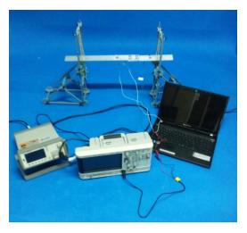
Figure 4. Experimental setup for guided waves measurements on the bolt-jointed aluminium beam.
