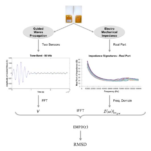
**Figure 1.** Overall procedure to extract the Damage Indicator based on Electro-Mechanical Power Dissipation.
