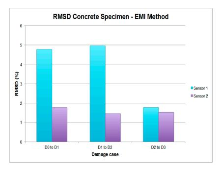
Figure 17. RMSD values for the concrete specimen corresponding to the EMI method.
