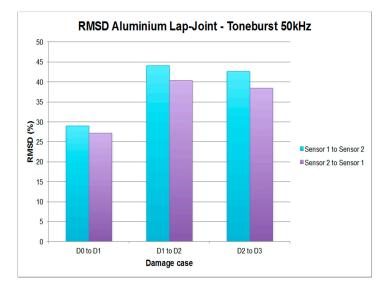
Figure 8. RMDS values for the bolt-jointed aluminium beam.
