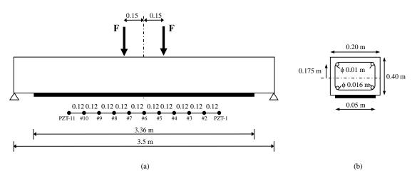
**Figure 18.** (**a**) Geometry, loading scheme, and sensor location map for the RC beam; (**b**) Cross-section of the beam.
