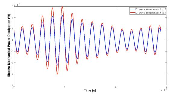
Figure 15. Differences in the EMPD in the concrete specimen for damage D1 when the wave travels opposite directions.
