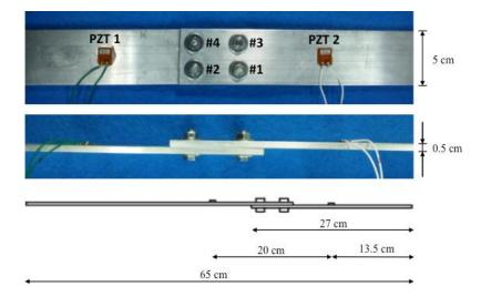
Figure 2. Bolt-jointed aluminium beam with two PZT transducers.
