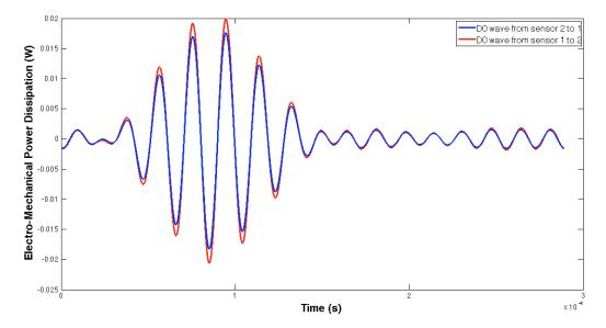
**Figure 7.** Differences in the EMPD in the aluminium lap-joint for damage D0 when the wave travels opposite directions.
