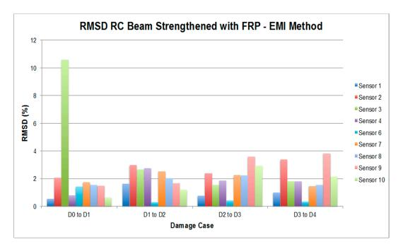
Figure 30. RMSD values for the RC beam corresponding to the EMI method.
