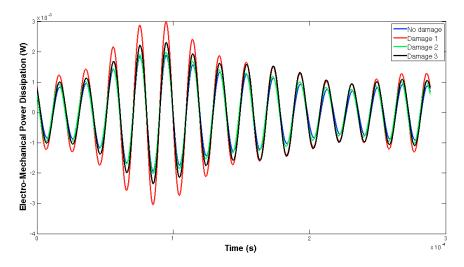
Figure 14. EMPD at 50 kHz. Tone-burst sent from sensor 2 to sensor 1.
