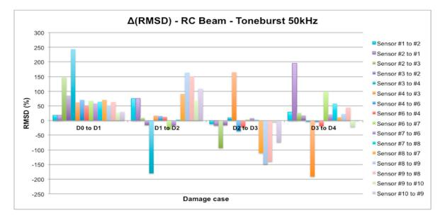
**Figure 32.** RMSD increments between loading steps for the RC beam corresponding to the EMPD method.
