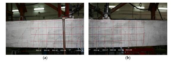
Figure 28. Cracking map of the beam after the last loading stage. (a) Left side of the beam; (b) right side of the beam.
