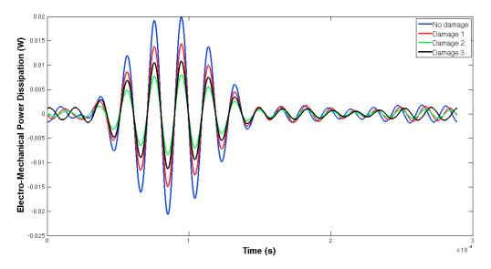
Figure 5. EMPD at 50 kHz. Tone-burst sent from sensor 1 to sensor 2.
