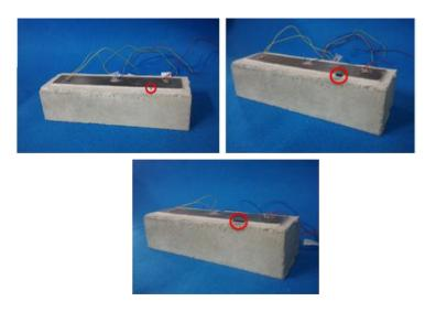
Figure 12. Damage scenario for an FRP-strengthened concrete specimen (II).
