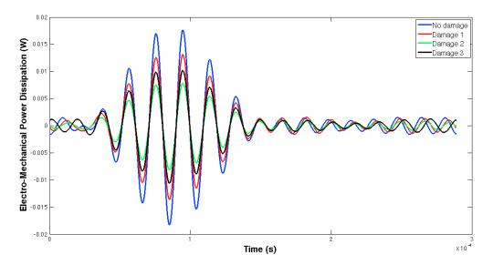
Figure 6. EMPD at 50 kHz. Tone-burst sent from sensor 2 to sensor 1.
