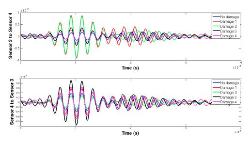
Figure 22. EMPD at 50 kHz. Tone-burst sent and measured between sensors 3 and 4.
