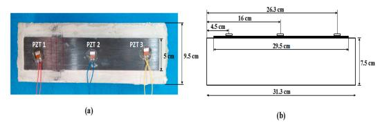
Figure 10. FRP-strengthened concrete specimen with three PZT transducers.
