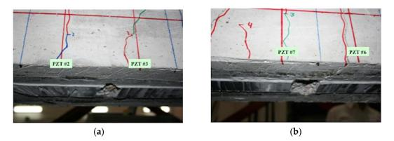
**Figure 31.** Damages with concrete cover separation between sensors 2 and 3 (**a**) and sensors 6 and 7 (**b**) for the RC beam.
