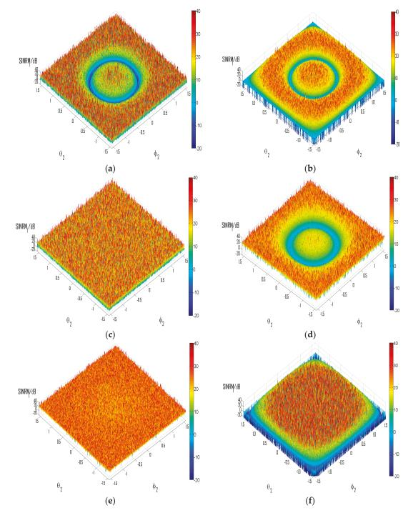
**Figure 10.** Separation performance of typical ICA algorithm under varied scenarios. (a)  $\beta = 2, D = 3$ ; (b)  $\beta = 2, D = 1.5$ ; (c)  $\beta = 0.7, D = 3$ ; (d)  $\beta = 0.85, D = 1.5$ ; (e)  $\beta = 2, D = 8$ ; (f)  $\beta = 2, D = 3$ .
