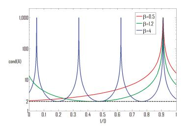
Figure 4. Condition number vs. the divergence of carrier frequencies.
