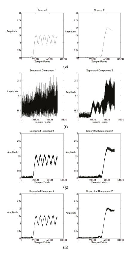
**Figure 12.** Restitution quality with the proposed scheme. (a) Original Sources (b) Recovered components, without extra phase delay (c) Recovered components, k = 1 (d) Recovered components, k = 2 (e) Original Sources (f) Recovered components, without extra phase delay (g) Recovered components, k = 1 (h) Recovered components, k = 2.
