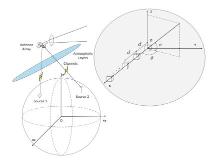
Figure 1. Spaceborne non-cooperative communication with antenna array.
