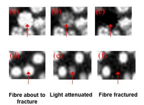
Figure 7. (a-c) Identification of imminent fibre fracture by monitoring the transmitted light intensity for a SDOF (a,d): whilst the sample was loaded in tension; (b,e) just prior to fracture; and (c,f) immediately after fibre fracture.
