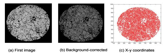
**Figure 5.** (a–c) Illustration of the analysis steps involved with processing the images obtained via the high-speed camera: (a) image from the high-speed camera at t = 0 (first image); (b) background-corrected image using Matlab<sup>TM</sup>; and (c) x-y plot for the location of the individual fibres.
